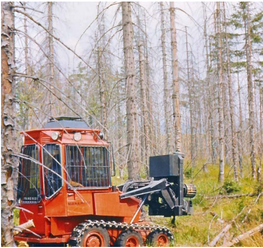
Lokomo Makeri 34T with felling scisors was used massively in Ore Mts. in the 70's.
