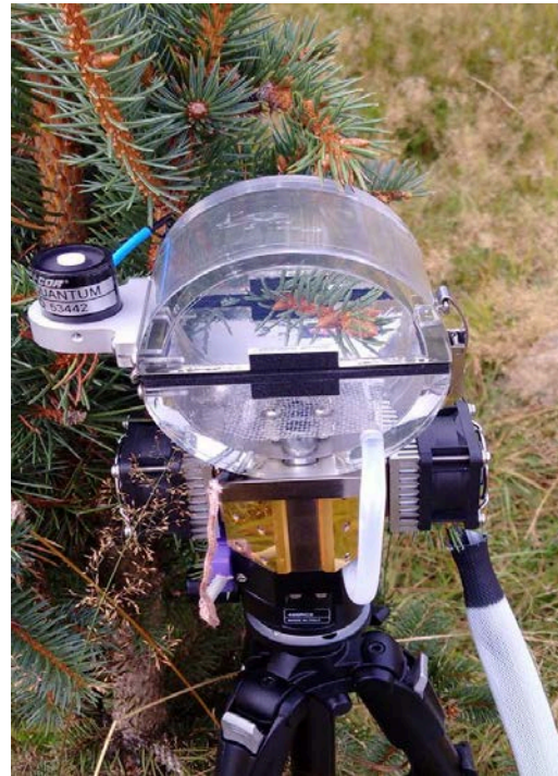
Gasometric measurement on blue spruce in order to estimate the photosynthetic parameters of individuals infected by the fungi.
