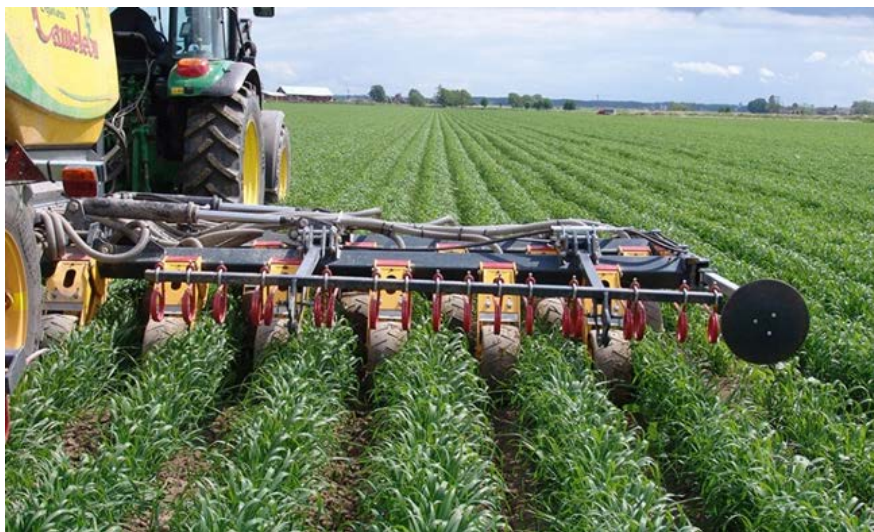
Image 28 – Parallelogram design of System Cameleon.
