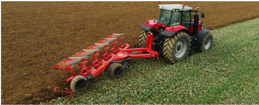
Image 16 – Shallow mould-board plough.
