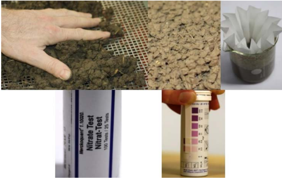
Image 6 – Steps of simple nitrate analysis.
