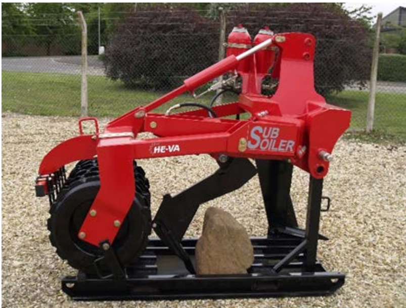
Image 13 – Subsoiler equipped with an air seeder during cover crop establishment. Source: https://twitter.com/HEVA_uk/status/1172171859523231744/photo/1
