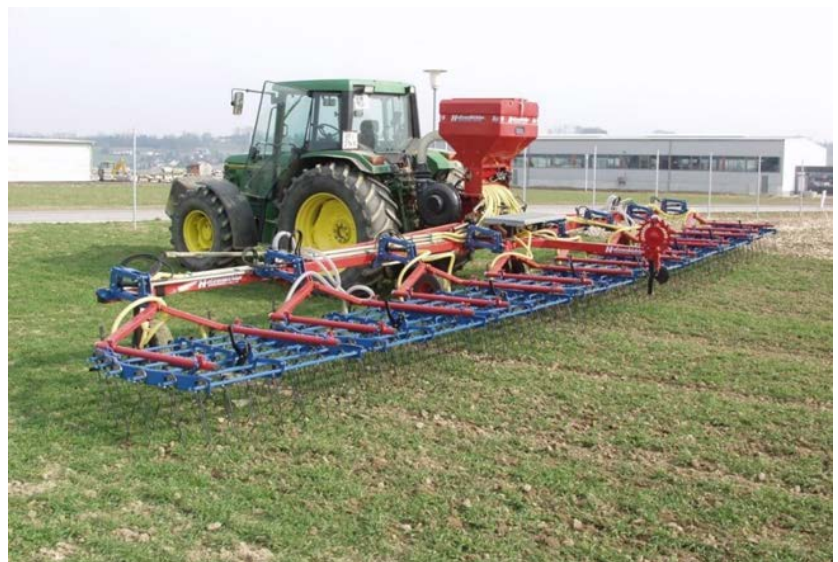
Image 24 – Tine harrow equipped with an air seeder. Source: https://www.hatzenbichler.com/en/original-harrow
