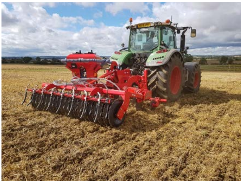
Image 13 – Subsoiler equipped with an air seeder during cover crop establishment. Source: https://twitter.com/HEVA_uk/status/1172171859523231744/photo/1
