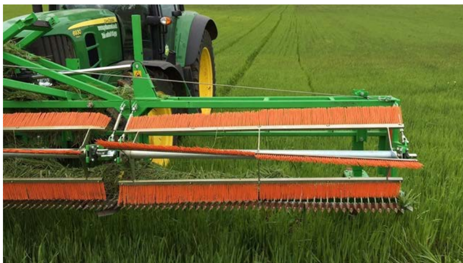
Image 29 – Combcut® during mowing weed. Source: https://www.primewest.co.uk/combcut/
