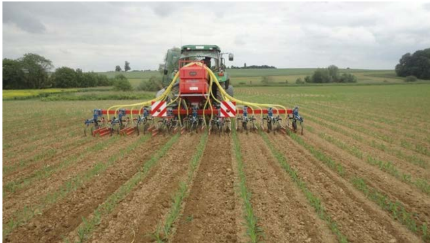
Image 27 – System Cameleon - a drill and interrow hoe in one machine. Each hoe is attached to a parallelogram to cope with terrain. It is equipped with a camera steering assistant and capable of undersowing cover crops during hoeing.
