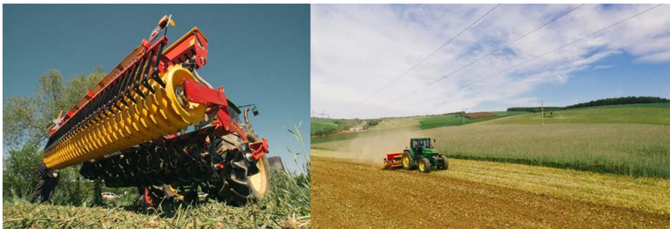
Image 17 – Passive disc implement for shallow cultivation of stubble or mulched biomass into the soil. Photo: Martin Matěj
