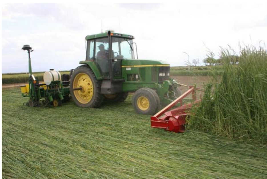
Image 20 – Roller crimping and drilling cash crop in a single pass.
