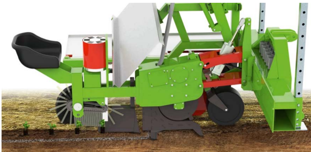
Image 34 – MulchTec, a solution for vegetable transplantation into high cover crop residue with a PTO driven slicing mechanism. The transplanter is also equipped for application of organic zone fertilizer.
